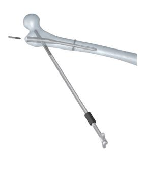
Remove Femoral Hip Compression Screw-B
